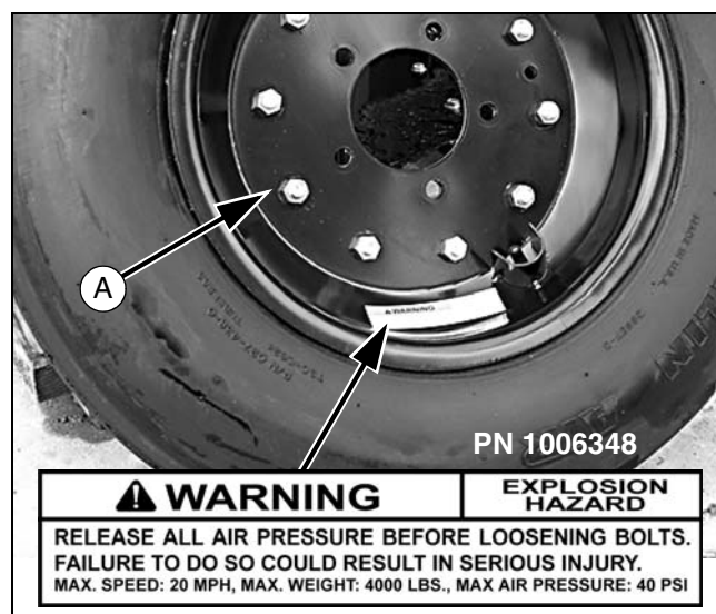
Figure 23. Split Rim Tire Servicing
